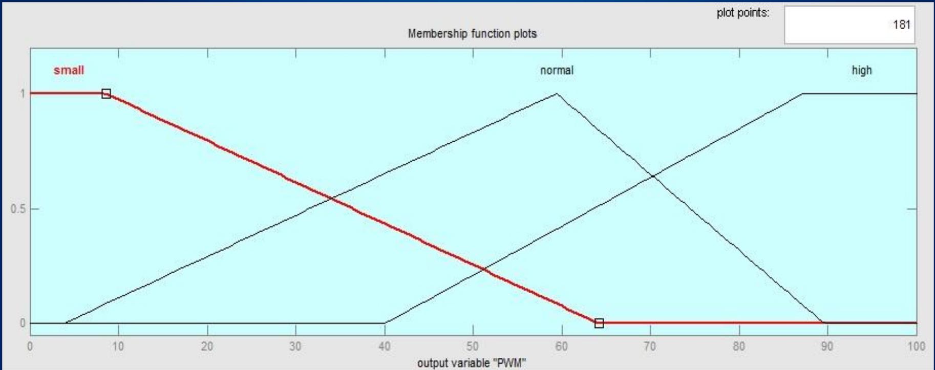
Output variable “PWM Peltier elements A”
